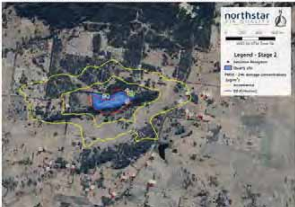
Figure 14 Predicted Incremental Maximum 24-hour Average PM 10 Concentrations – Stage 2
