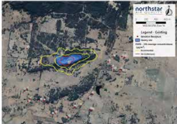
Figure 13 Predicted Incremental Maximum 24-hour Average PM 10 Concentrations – Stage 1
