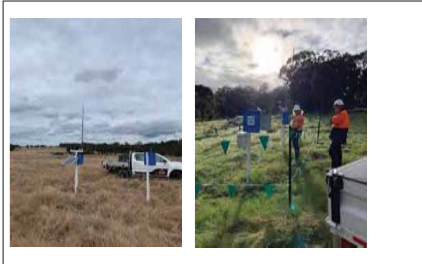
Figure 3: PM 10 /PM 2.5 Monitoring gauges and data transmitters
