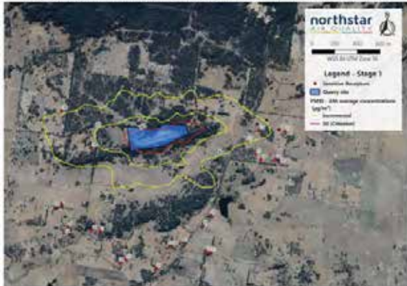
Figure 14 Predicted Incremental Maximum 24-hour Average PM 10 Concentrations – Stage 2
